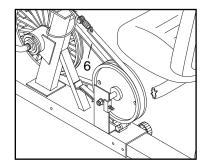
be removed. Refer to the instructions on this page and remove the left and right side shields. Next press down on the center of the Drive Belt (6) between the front and rear pulleys. There should be from 1/4" to 1/2" of vertical movement in the center of the Belt.
